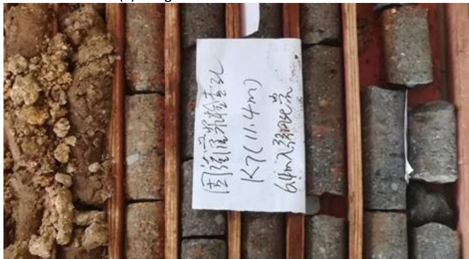
(b) A geological log record at Karimenu II Dam site laboratory
